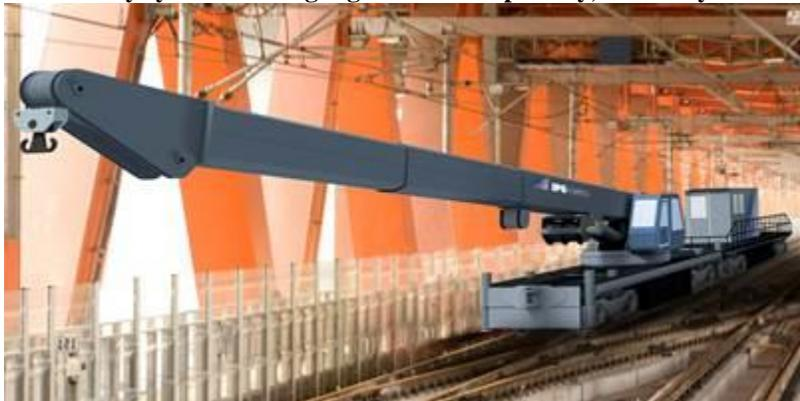
Duluth, MN. - We are pleased to announce that IPS Worldwide is expanding into the Metro Railway System with the introduction of our new IPS Metro Crane. The Metro Crane is an emission free railway track crane used for maintenance of the underground rail systems. Currently, IPS Metro is the only company in the United States that has the ability to manufacture this type of crane.
